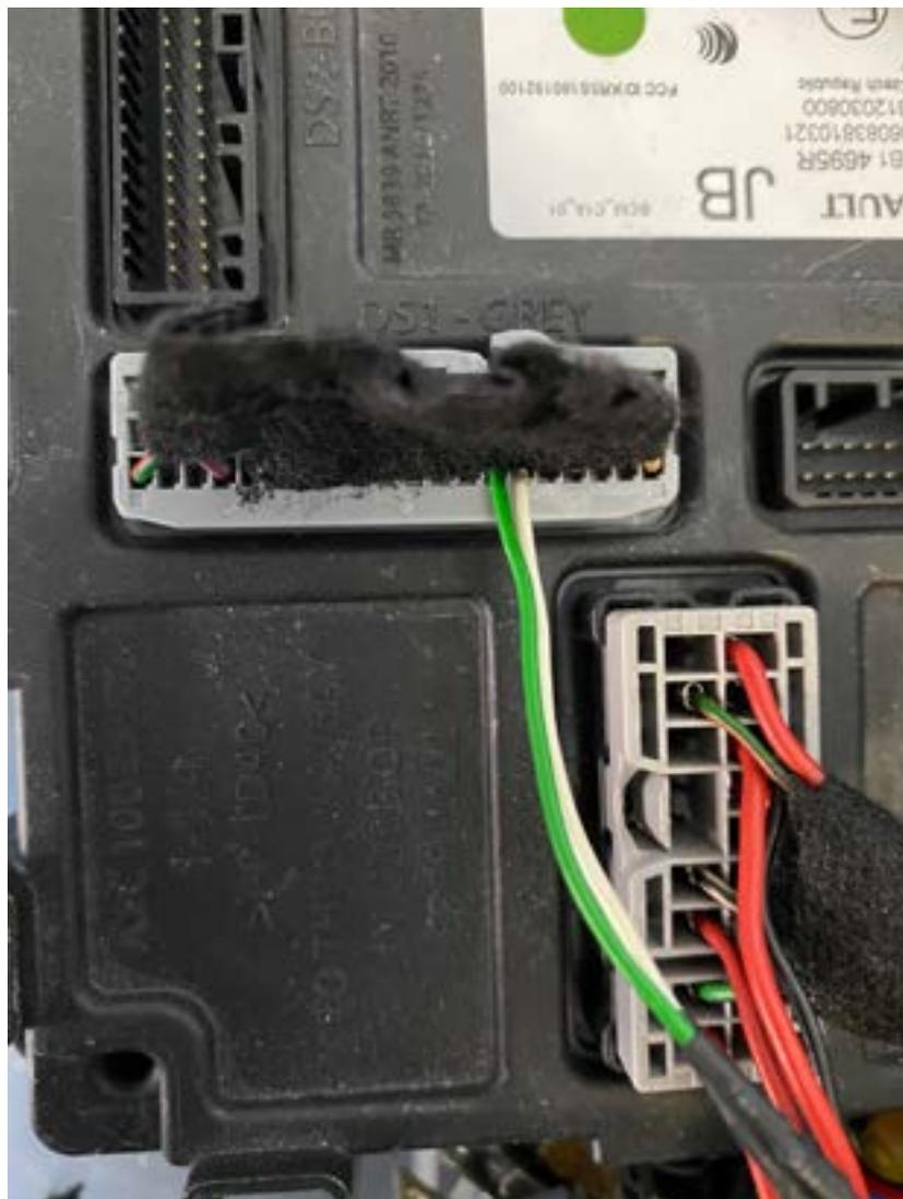
Important : The new generation UCH (SWEET 400) requires CB012 connection by attaching the needles to pins 2 and 3 of the green connector.
