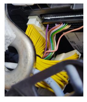
Pictures below show the connections to BCM (UCH) Unit of New Zoe, where the unit is located above the pedals:
