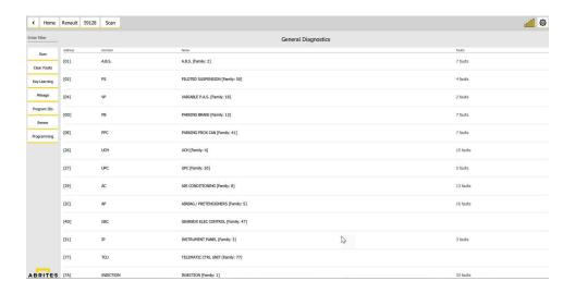
After you see the list of modules you can enter each of them in order to do diagnostics: Read DTCs, view live data, perform actuator testing and so on. You can monitor live values in a graph form (with live graphics being displayed) or using the table view of the software to monitor as many parameters as you wish simultaneously:
