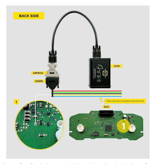
**Important:** Be careful and make sure you work with the module according to the wiring diagrams. Front and back sides are important to distinguish and solder the correct wires to the relevant sides, as well as remove the correct components, then return them to their places.
