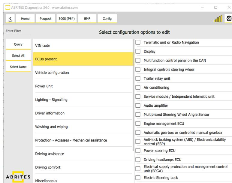
In this particular case we can add a passenger compartment air blower to be added to the passenger compartment of the this P84 3008
