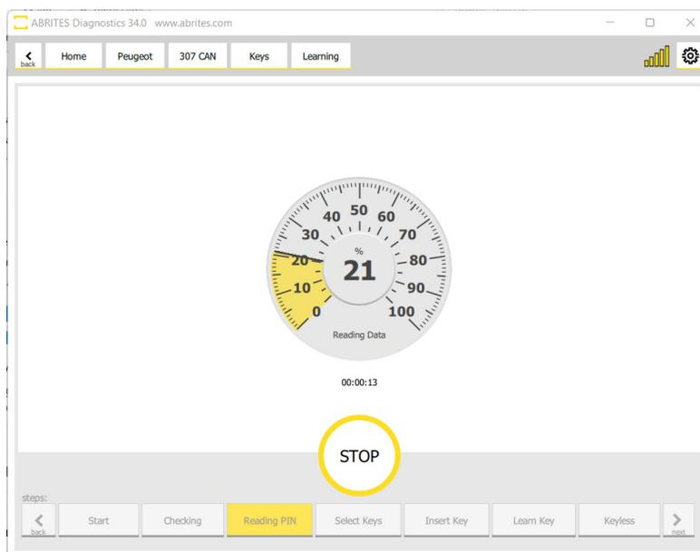
After the procedure for reprogramming the BSI is completed you will see the pin code.
