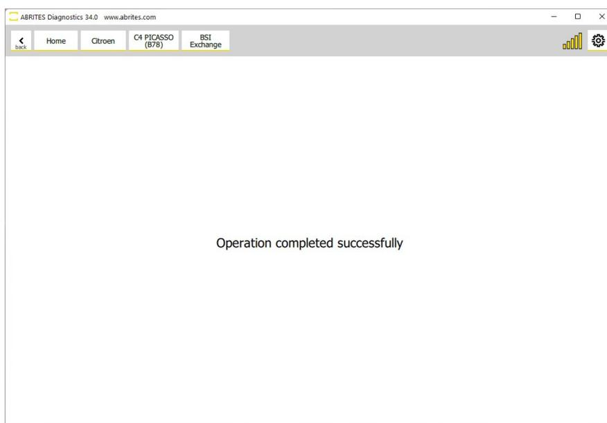
4. After the file is saved you are done with the old BSI module and you can install the new one in the vehicle.
