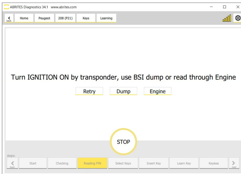
If you decide to load a dump of the BSI, you can read it by soldering to specific points of the unit, and reading it on bench. You will need an [ZN030 Abprog programmer](#), and a [ZN057 Wire Extender](#) for Abprog
