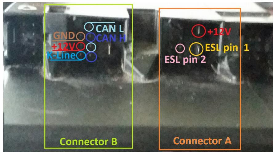
W220 / W215. Here the connectors are two A and B:
