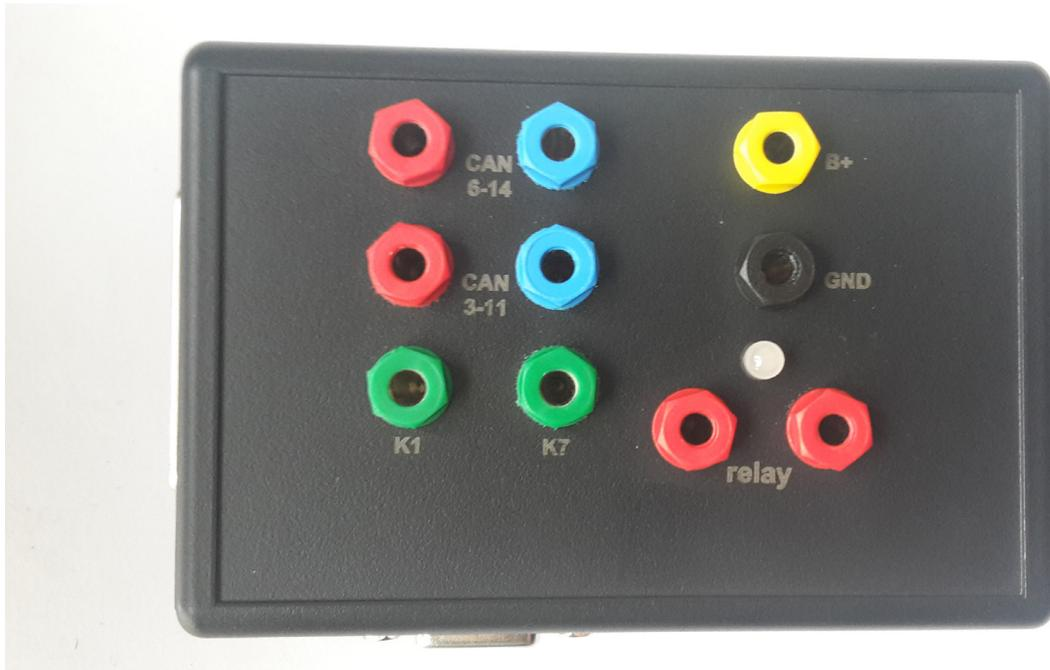
1st two ports (Red and Blue) are for CAN HI and CAN LOW 6-14, the 2nd ports below them are for CAN HI and CAN LOW 3-11. These ports are mainly used when virginizing and adapting Mercedes TCUs and ECUs when using MN026.
