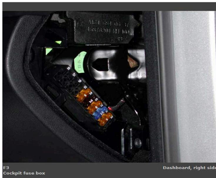
W164 passenger fuse box. EZS fuse is socket 14
