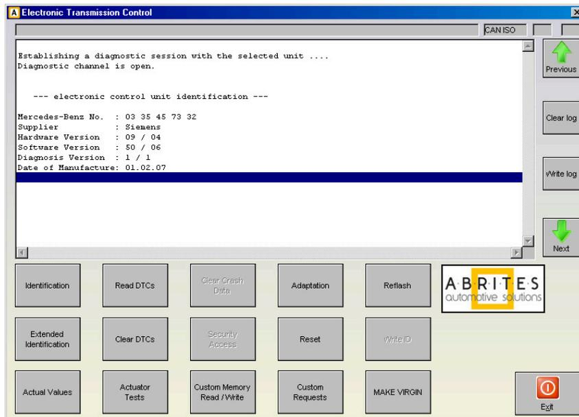
3. Pressing the button “Adaptation” will show the available adaptations including the SCN coding string. You may save the SCN coding string from a damaged control unit and then you can save this saved SCN coding in the donor 722.9 control unit:
