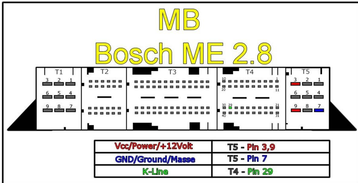
EIS/ EZS connection pinouts for bench connection.
