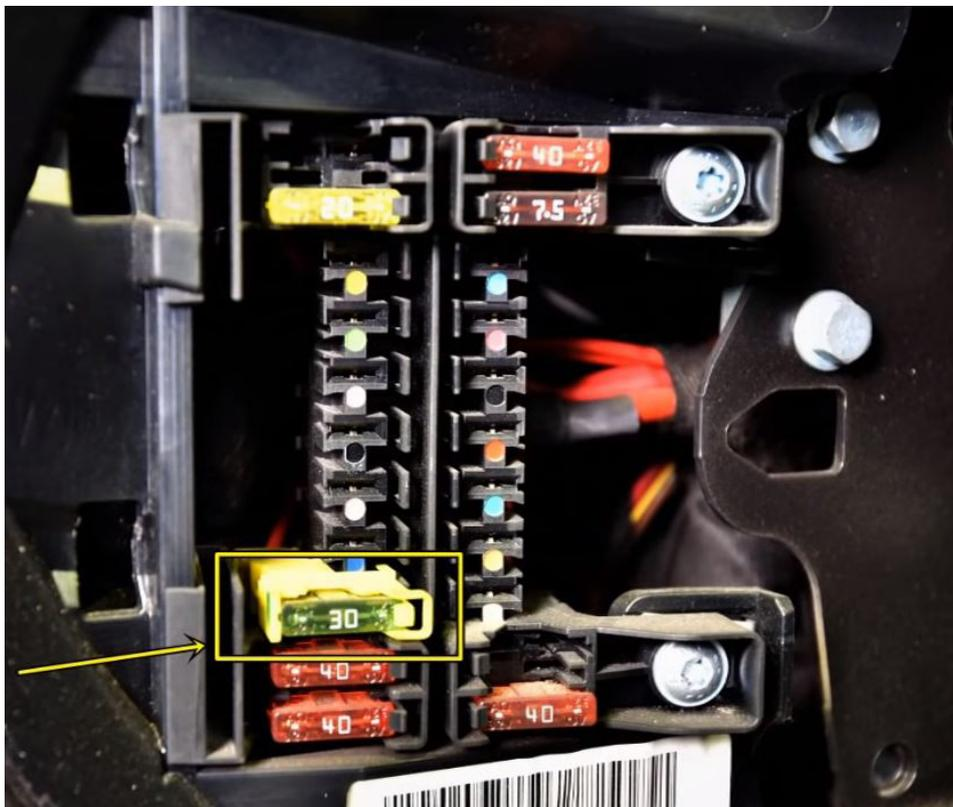
W164 EZS fuse can be found on socket 14 in the passenger side fuse box.
