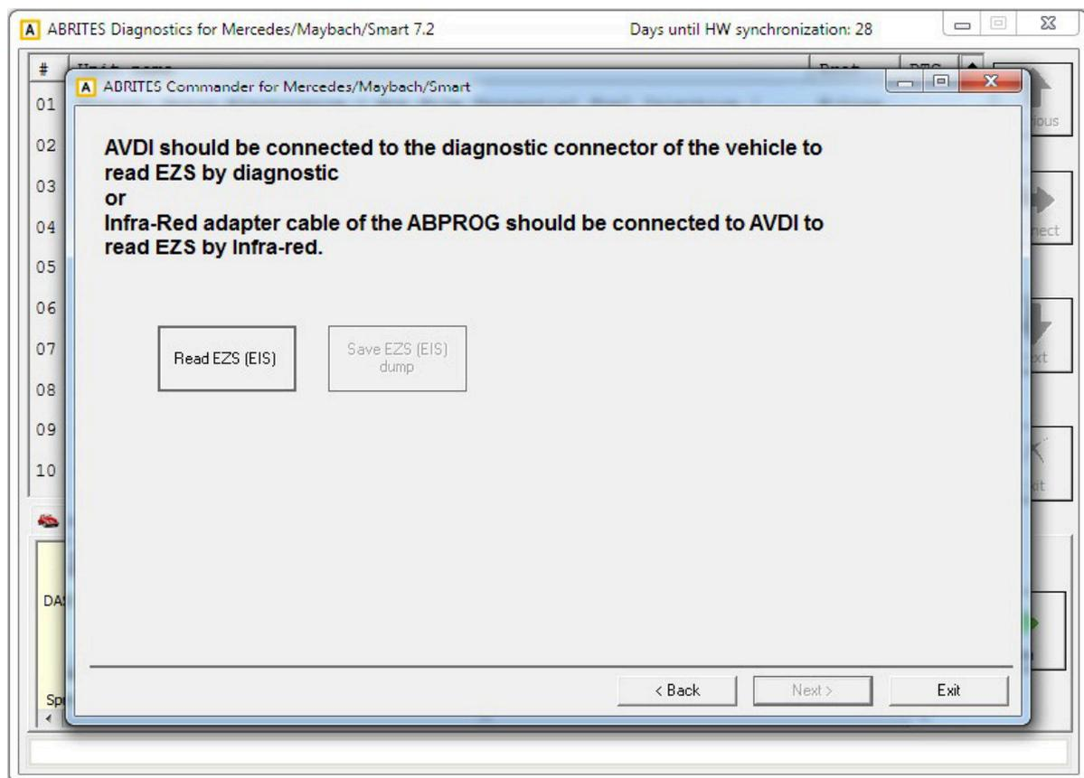
At this point the software will explain what needs to be done in order to read the EZS (EIS) dump either by OBD or by the IR adapter.
