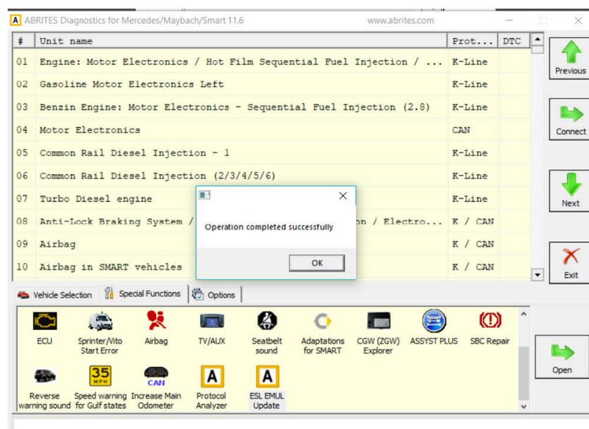
To determine the software version of the emulator, you need to have it connected on bench or the car. Toggle switches must be set as if working with a W204.
