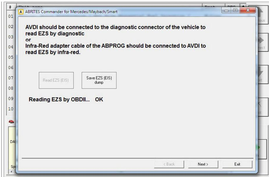
The EZS (EIS) Configuration data reading completes with success and you can now save the dump using the “Save EZS (EIS)” button. Once you have the EZS (EIS) dump you can proceed to the next step. This is where the password for key learning needs to be extracted. This is done in the following manners:
