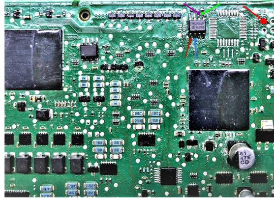
The photo below shows how to connect to a BMW BDC and a FEM unit to read the EEPROM:
