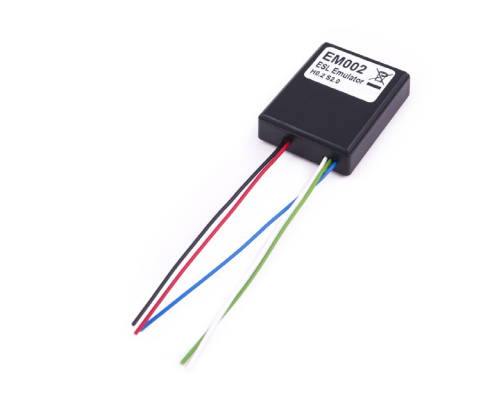
EM002 - ABRITES ESL EMULATOR FOR RENAULT
