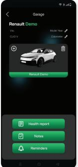
**The Garage button** opens the virtual garage, you can save your favorite cars there manually, or check the option to automatically add all scanned vehicles inside. You can access Virtual Garage anytime, without need to use or connect your MODI device.
