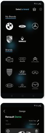
**The DEMO button** works to show you a basic example of how the application works without the MODI device, you can also use generic OBD2 option when you connect to the MODI device option where you can use it without subscribing for the application. With Generic OBD2 you can scan few modules of the vehicles, read and clear DTCs.
