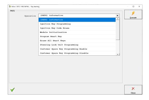
When programming smart keys, for example, you need to select the appropriate option from the drop down menu and press the button "Execute". The procedure would continue with on-screen suggestion messages on what needs to be done on you side.
