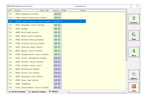
From the first screen you can select the vehicle you are working with, do a Scan for Units (and DTCs) and Clear DTCs. Also, a sub-menu with options is available from this screen.
