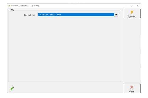
Please follow the on-screen instructions and once asked, insert an new (unlocked) key in the key slot. The number of the keys on screen must increase once the key is programmed. New key ID will appear in the screen log. The CEM accepts only unlocked HITAG2 transponders. Once you programm all the keys that you wish ( you need to see the number as in the second picture) you can stop the procedure and keys should already be successfully programmed and you can see it in the logs sreen behind.
