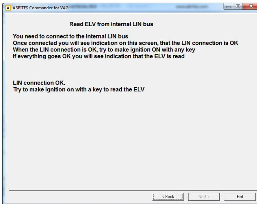
So once you have connection to the line, you should try to make several times ignition ON and again OFF (during these attempts you need to eject the key). Continue to make ignition ON and OFF with the key which you prepared on step 2, until you see the message "ELV read OK". Then you can continue with the next step.
