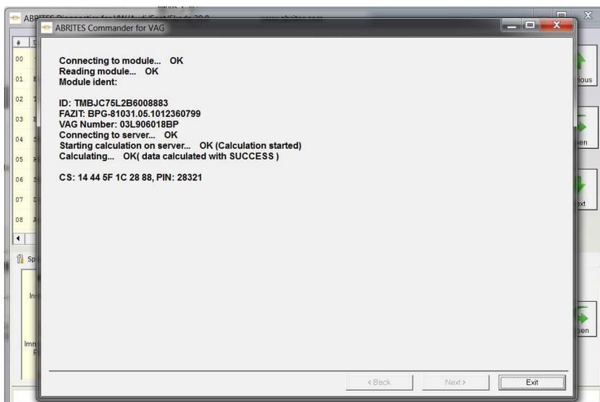
You can use later the PIN/CS for key-learning, or for adapting the ECU/TCU to the car
