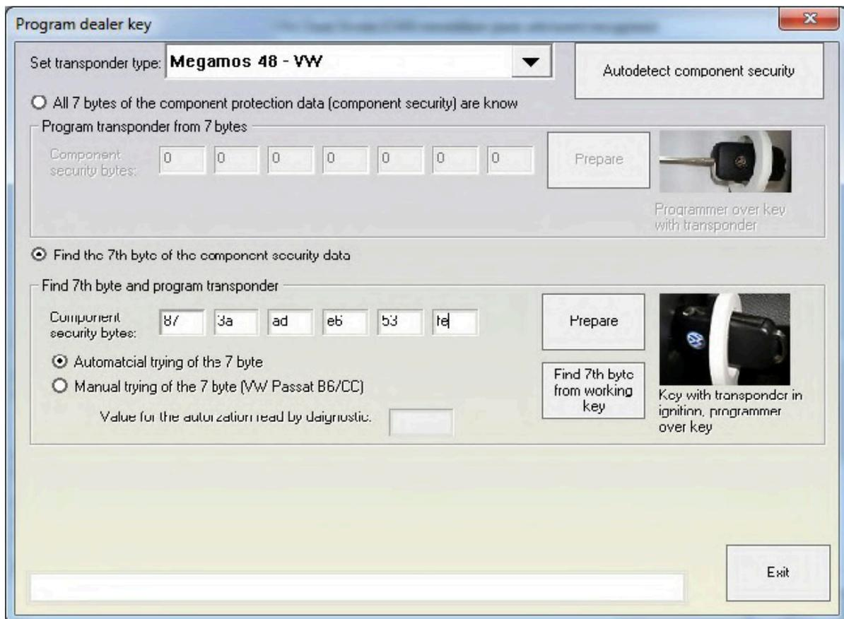
The 7 bytes of the component protection data are contained inside the immobilizer and sometimes inside the engine control unit. Inside the engine control unit there are always at least 6 of the component protection bytes stored, sometimes also the 7th byte is contained.
