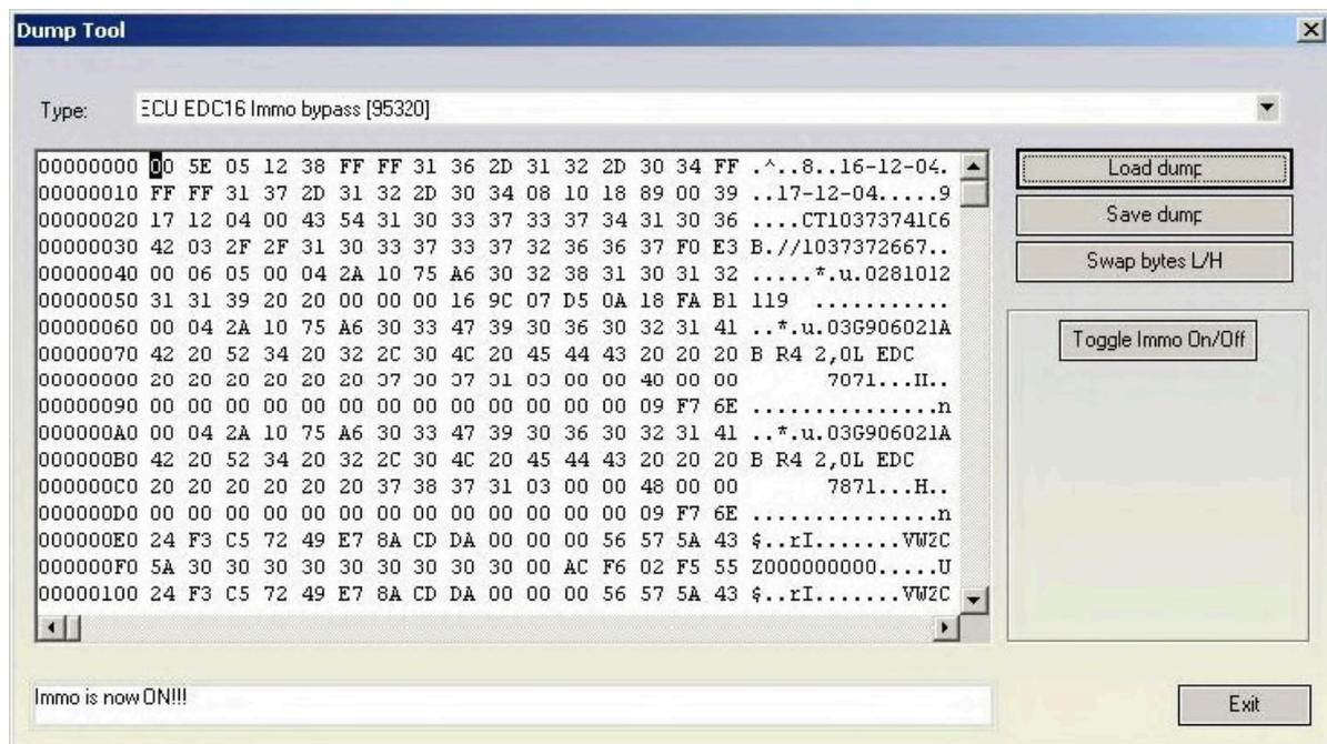
The “Toggle Immo On/Off” button allows to switch on/off alternatively the bypass function.
