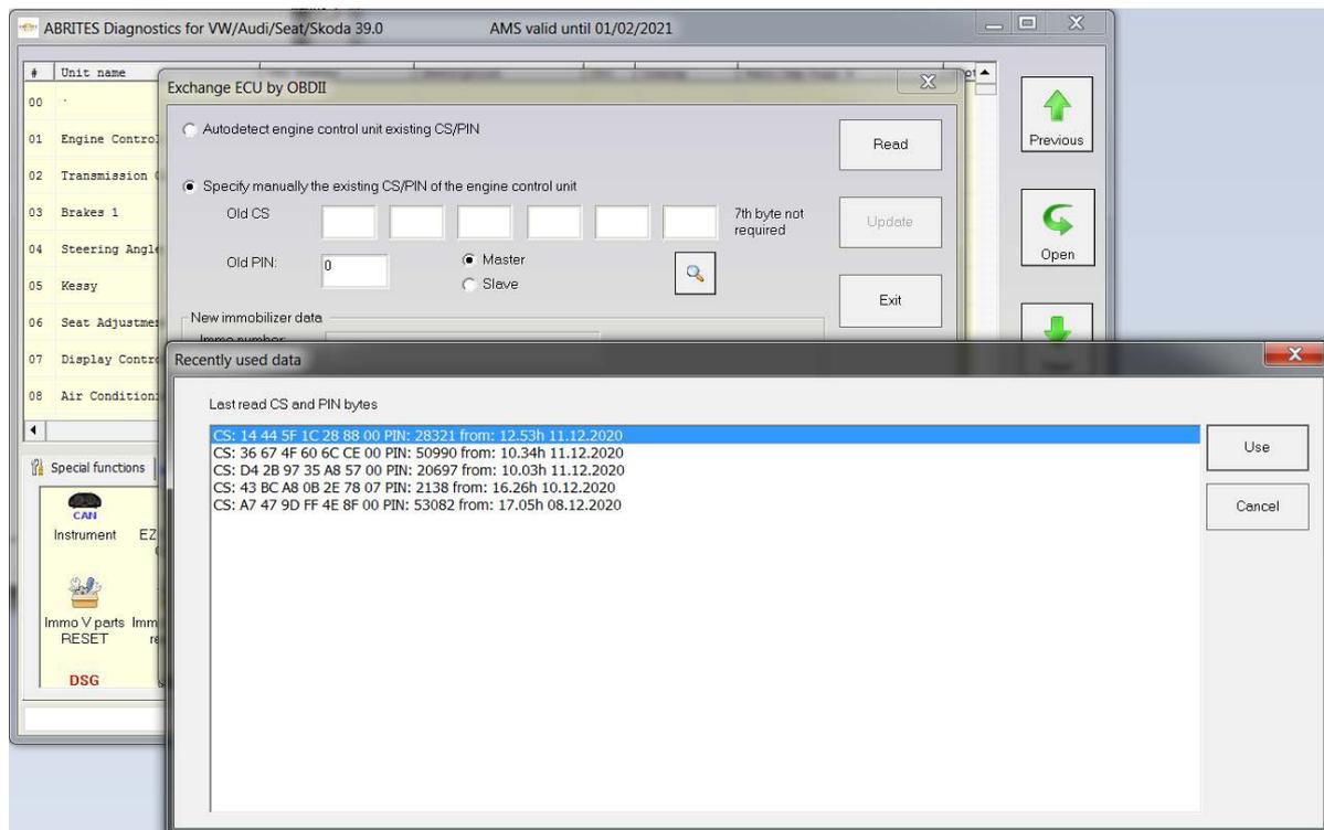
**IMPORTANT:** If the module (engine control unit or transmission) is not in its original state (e.g. the PIN/CS were already changed with some after market tool), the calculated data might be wrong.
