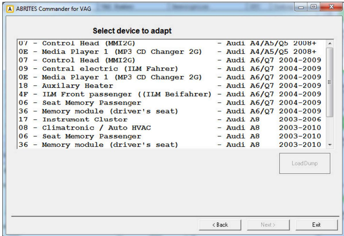
Currently for most of the modules it is needed to read the internal EEPROM (for the MP3 CD Changer the internal flash) with a programmer first. If it is not necessary to read the flash, the “Load dump” to read flash or EEPROM will not be active and the user can proceed with the next step.
