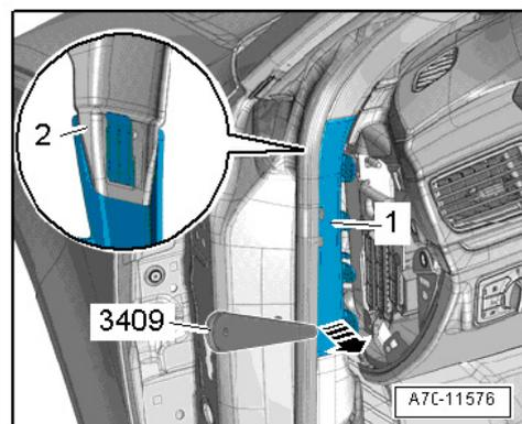
1.2 Unclip trim cover -1- for A-pillar (bottom) using removal wedge -3409--arrow- and detach downwards from A-pillar trim (top) -2-.
