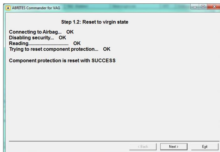
After the operation is completed the module is in a virgin state and can be adapted to any car.
