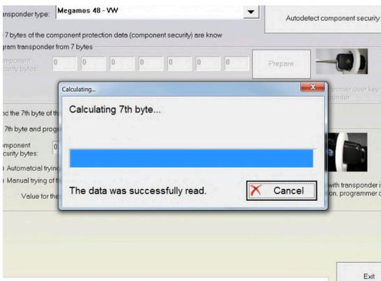
9. The 7th byte was found and you will be prompted to insert either a transponder or a blank key into the programmer to program it:
