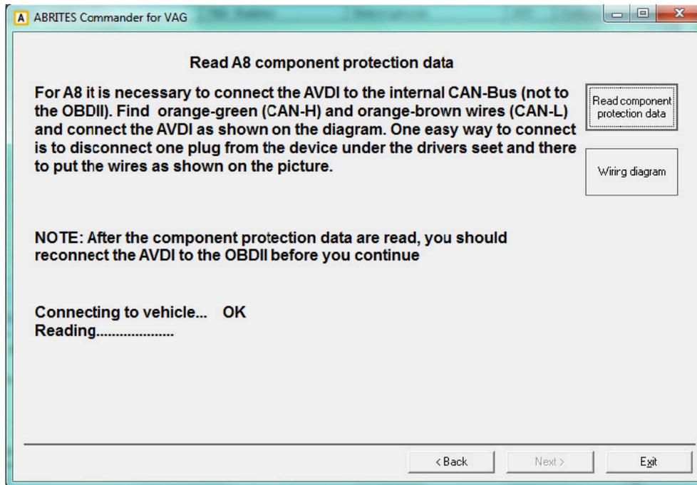
After the component protection data are read, you can continue with the adaptation.
