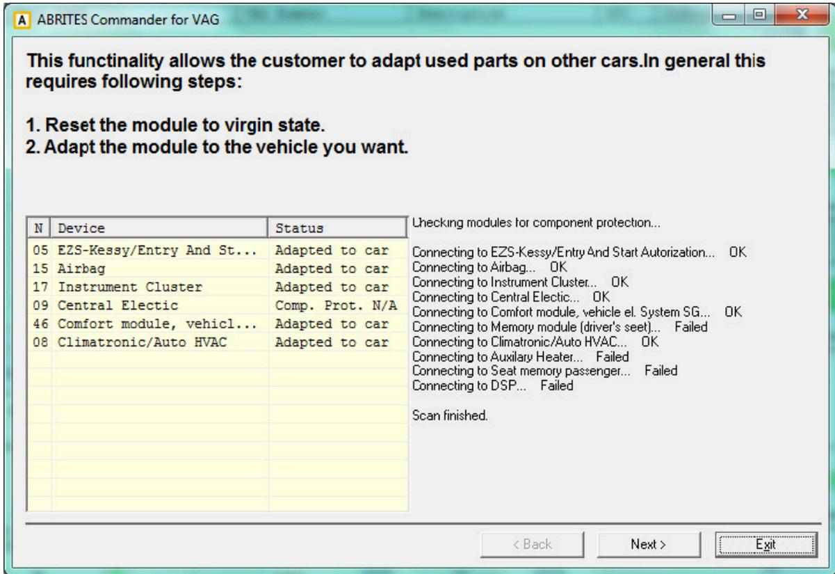
From the displayed list of available modules, the customer has to select the module which they want to adapt. Then the procedure of adapting the component protection is performed in two steps:
