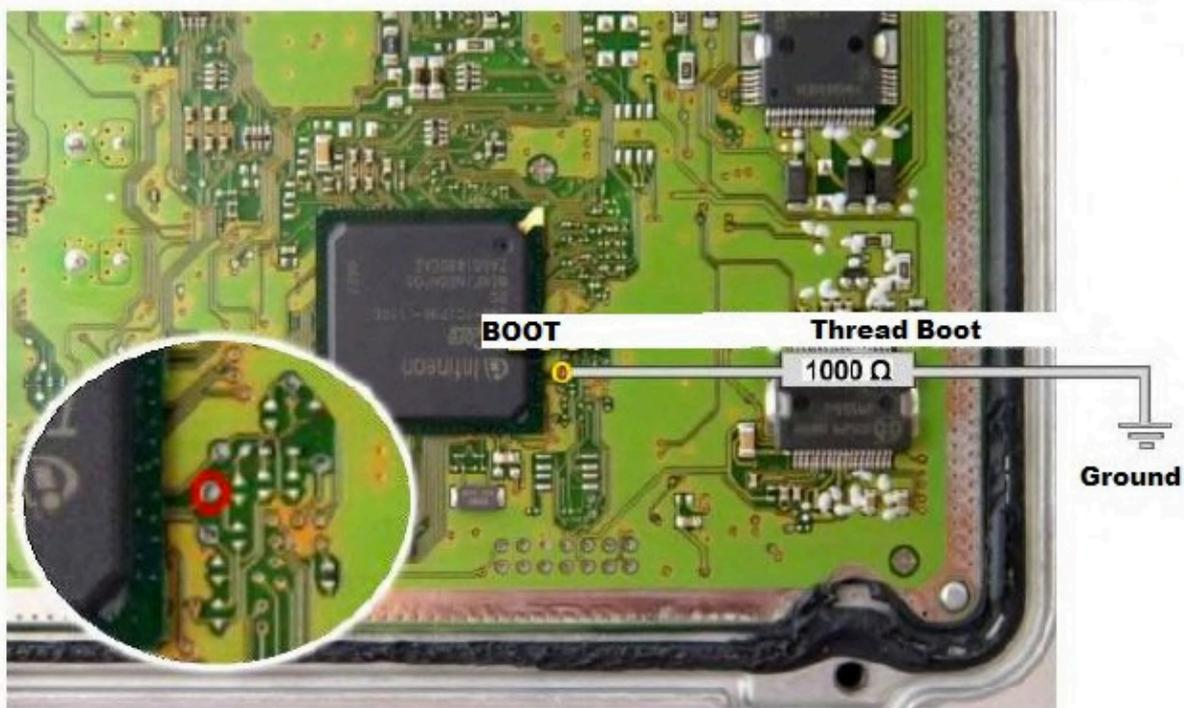
ECU Vag MED 17.5.1 – TC1796 with Internal and External Flash
