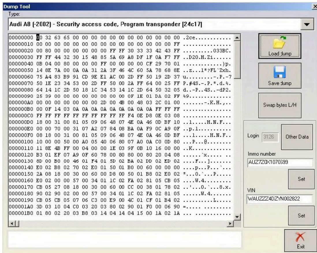
Pressing the "other data" button displays the learned keys and if a programmer has been recognized, allows to read current transponder's data and add it to the dump.
