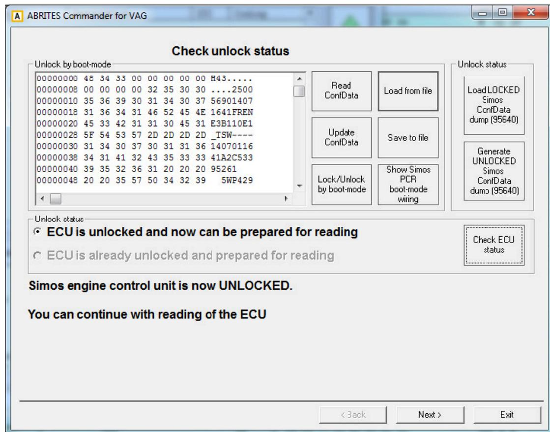
The procedure of reading the Simos PCR engine control unit consist of 3 steps:
