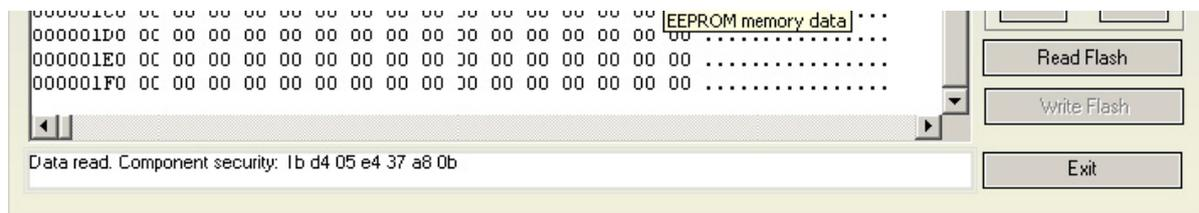
For CAN TP2.0 immobilizers in most of the cases it is possible to read all 7 bytes from the instrument/ immobilizer. This is possible from the Immo panel – you have to go to “Special function”, then “Instrument CAN” and “Read/write immo data”. After you read the immobilizer data in the field “Serial Key” the 7 bytes of the component security will appear.
