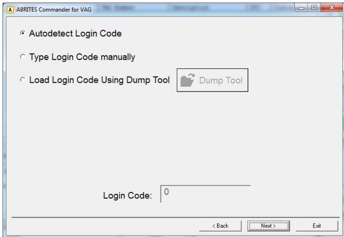
When the Login code is available and the "Next" button is pressed, an informational dialog is displayed, where the key recognition and engine start conditions are checked. The meaning of the fields is the same as the described in the standard key-learning mode.
