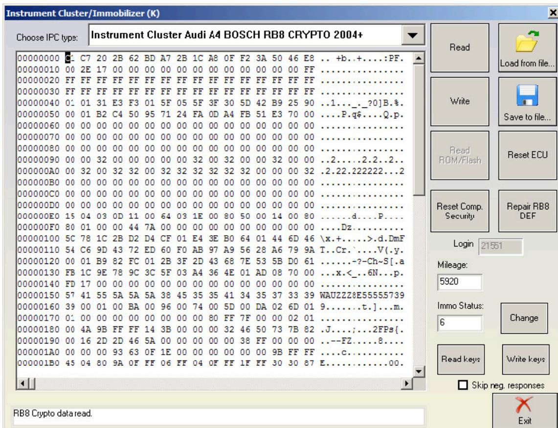
In order to transfer the keys you already have you have to first read the EEPROM of the source instrument and then by pressing the “Read keys” button you save them into a file.
