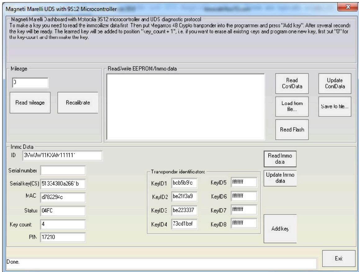
The special function is used for mileage reading and key making. Part exchanging and adaptation as well as identification and configuration is also possible. The mileage function requires a separate license while dealer key making requires the dealer key license.
