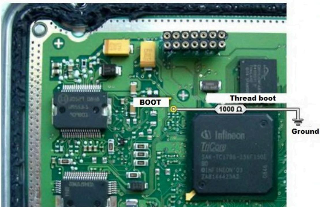
ECU Vag EDC17 CP24 – TC1796 with Internal and External Flash
