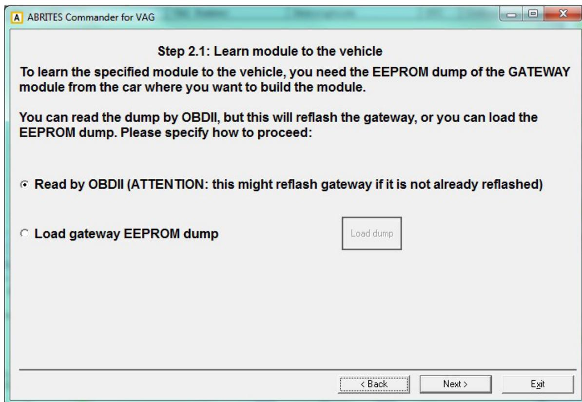
You have the option to read the Gateway EEPROM dump manually with a programmer, or to read it by OBDII. Reading by OBDII normally takes about 3-4min, but requires a module reflash. If the gateway is once reflashed, further operations of the EEPROM reading do not need a reflash.
