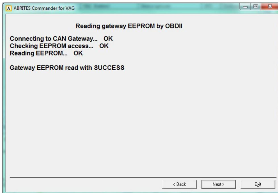
Once the EEPROM data are read/loaded, the adaptation of the component protection is performed. Once this step is completed successfully, the module should be fully functional.
