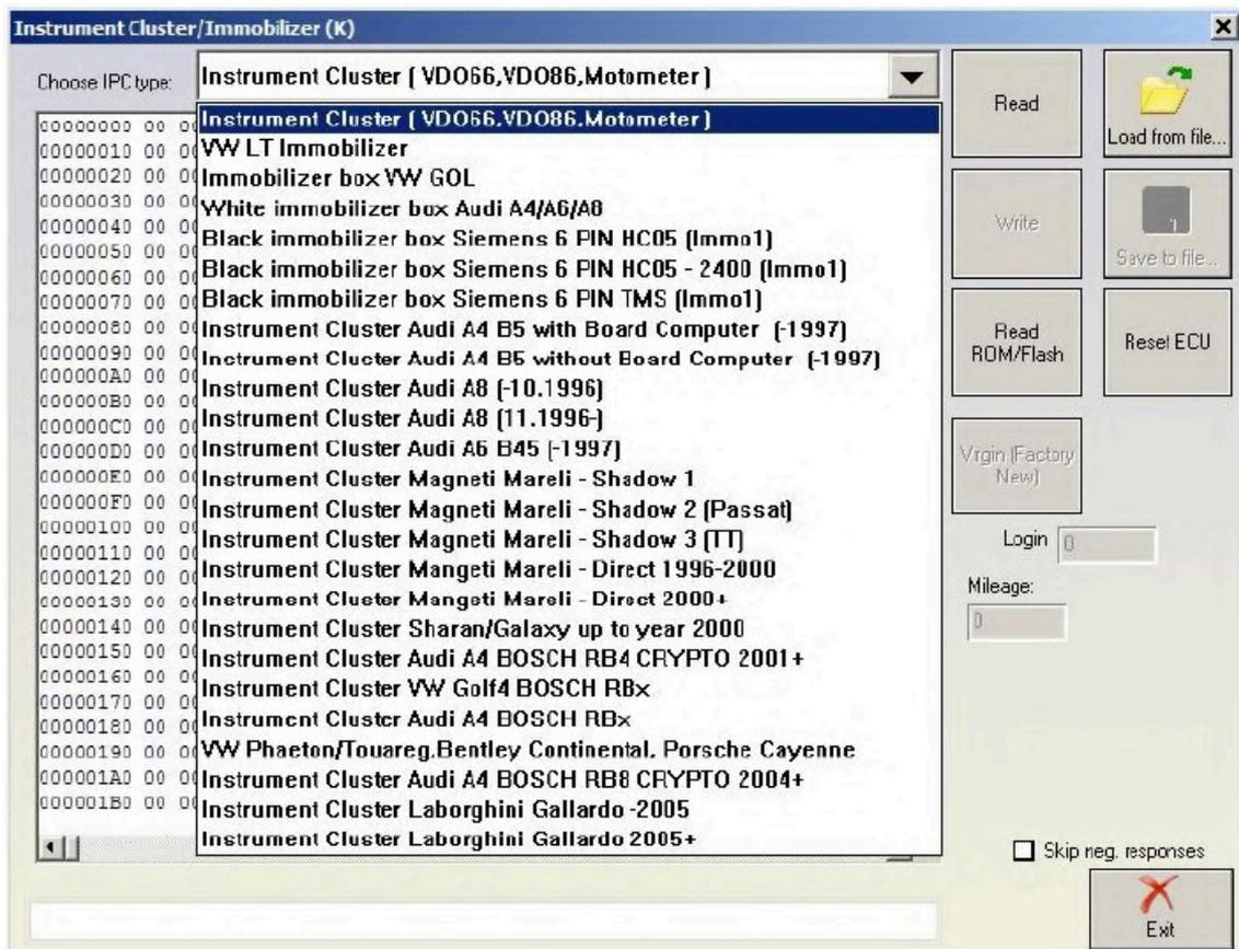
From this dialog box you will need to choose your instrument cluster type or the immobilizer and then you could read/ write the EEPROM ( read mileage, PIN etc.) Please be informed that the special function will only establish a connection via K-line ( KWP1281 or KWP2000) and this does not depend on the configuration options.
