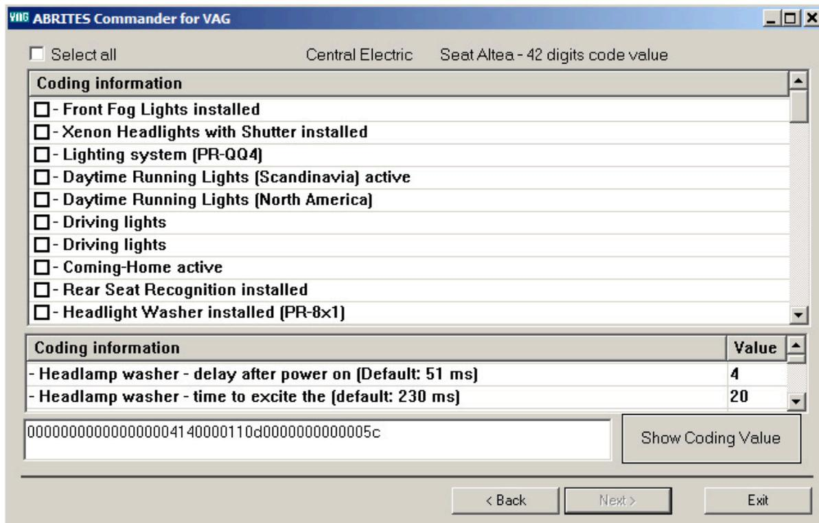
In the opened window you can check/un-check the desired features (see list with check-boxes in the above picture, modify certain value (see the list with the two columns (text and value) in the above picture) or select certain value by combo-box selection.
