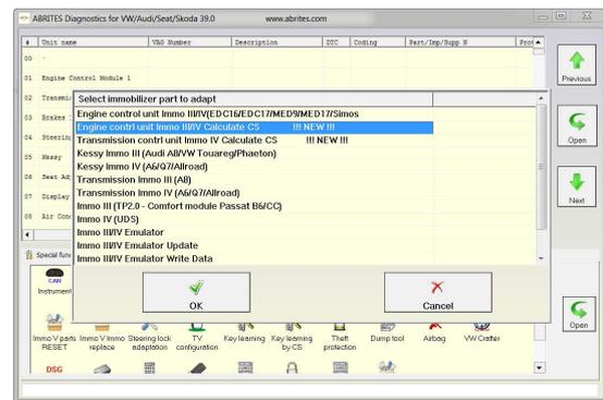
You can read the PIN/CS of the transmission control unit from special functions > Immo 3/4 parts adaptation > Transmission control unit Immo 4 calculate CS
