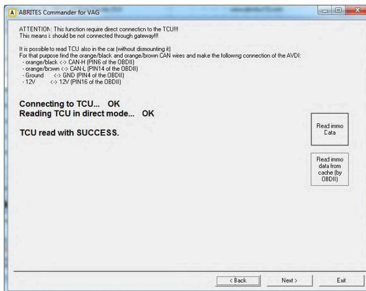
On the first step you need to read the TCU (with the connections described above). Once the TCU is read, you can connect the AVDI to the OBDII and proceed with the adaptation. Here is possible to use the so called "read from cache" which reads actually from the cache memory the last successfully read data for this TCU.
