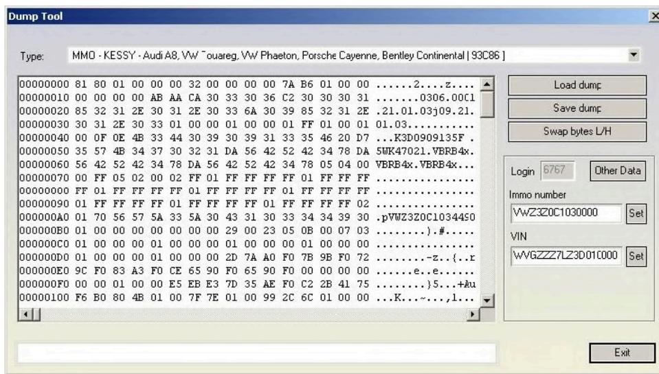
Pressing the “other data” displays the learned keys and also allows changing the immobilizer status (on some models changing the immobilizer status is used to put the Kessy e.g. into delivery condition).
