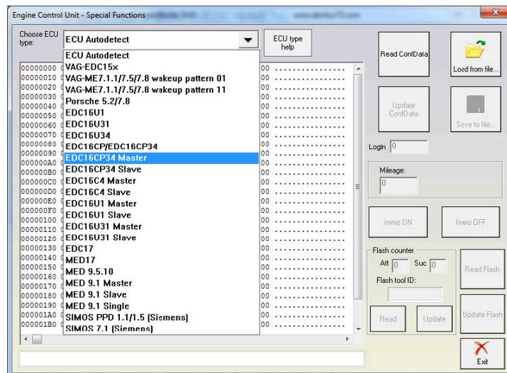
**IMPORTANT: You need to specify the type of Engine Control Unit in the car before proceeding! There is also an “Auto detect function” implemented which will detect the ECU type in almost all cases, however it is possible that it is wrong and then you need to select the type manually.**
