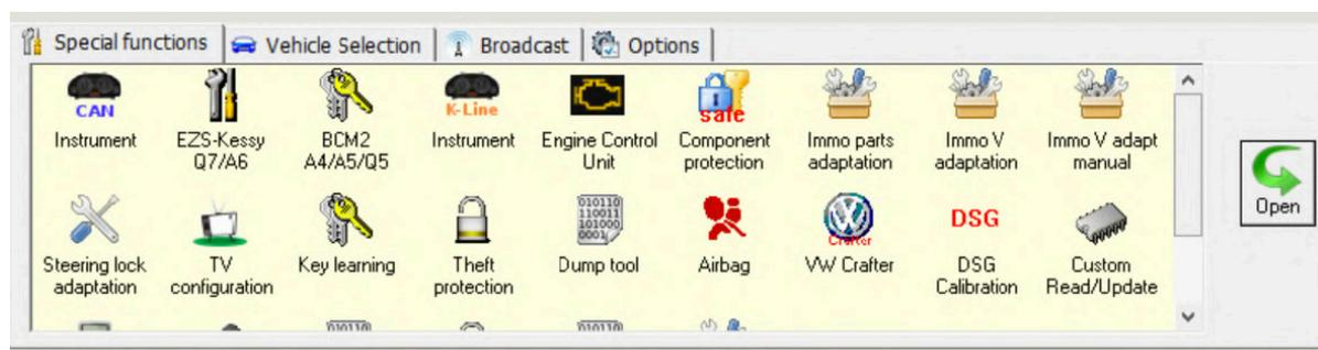
The needed special function is opened by double click or by marking and clicking the “Open” button.
