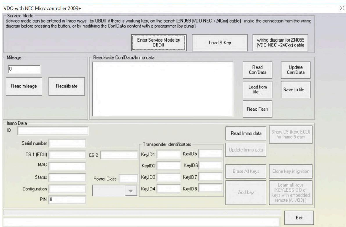
This special function can be used to read mileage and making keys. It is also possible to use it for exchanging parts and adapting the identification and configuration.
