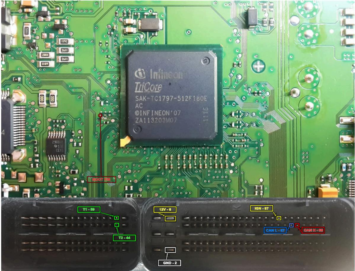
ECU MM\_9GV Pinout Diagram:
