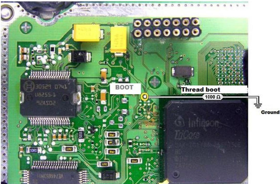
ECU Vag EDC17 CP14 CP20 - TC1796 with Internal and External Flash
