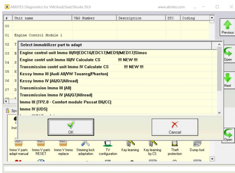
When the function is started, the connection to the control unit is established and the required data are read from there. It is necessary to have connection only with this module, not necessary to have the whole vehicle connected. I.e. this means that you can do this on the bench.
