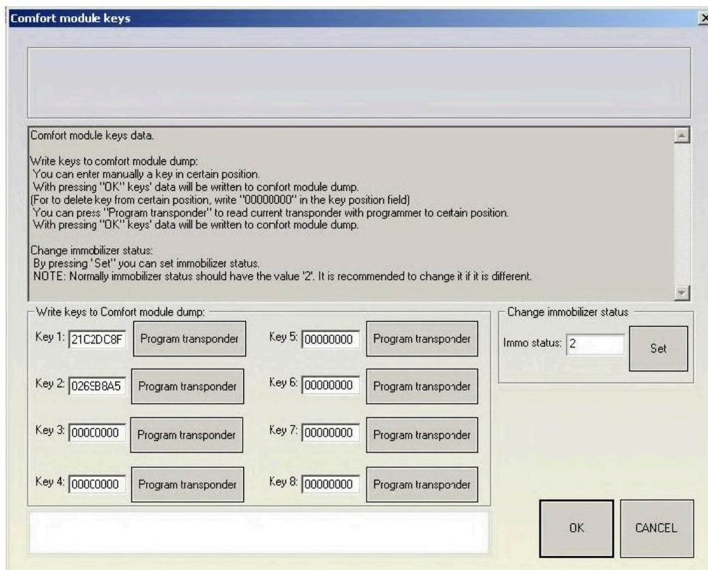
Keys with data “00000000” represent the empty positions in the dump file (position at which no key is learned). The rest are already occupied and represent the data of the learned at the respective positions keys.
