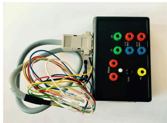
N.B! Please be informed the DB15 cable that is part of the Distribution Box set needs to be disconnected from the power supply during the wiring process of the unit if ZN051 is used.
