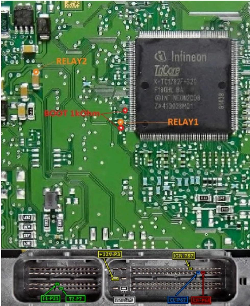
On Different EDC 17 ECUs, you can follow the following steps to connect to the ECU when using the ZN051 Distribution Box.
