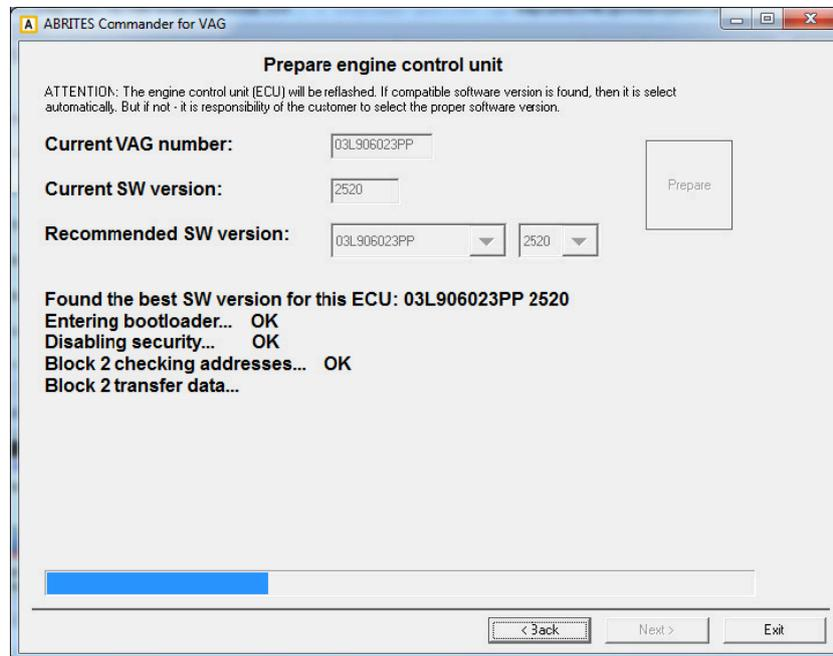
c) Once the engine control unit is prepared, the ECU can be read by OBDII. Once it is prepared, it is possible to proceed directly to the last step. It is also possible to read the PIN/CS/MAC from the “Immo parts adaptation” and “Engine control unit” special functions. But unlocking and preparing for reading can be made only from the “Simos PCR2.1” special function.
