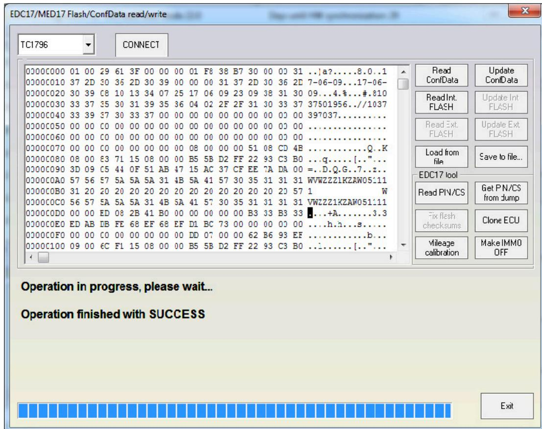
If the user presses “Read PIN/CS” the PIN, component security and MAC will be displayed:
