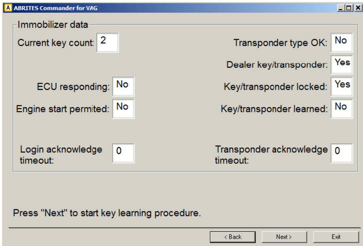
Pressing the "Next" button here will start the adaptation procedure and after finishing it the user should give ignition ON with all available keys.
