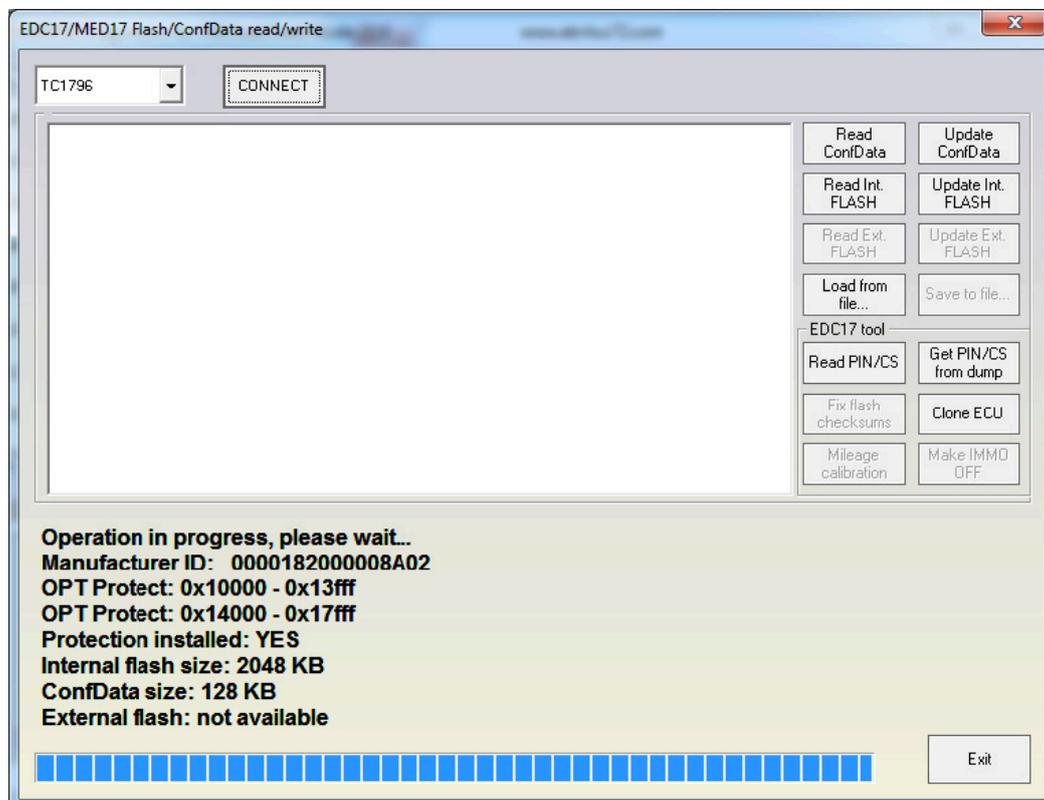
Then you should select the appropriate microcontroller and connect to it. Once connected the user has information about the flash/EEPROM size and protection, and has the ability to:
