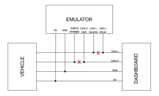
Below you may read about the different types of connectors you will find in the vehicles the emulator works for. PIN connections and wires' colors are described:
