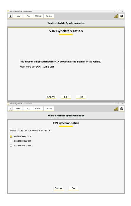
Proxi Alignment is needed after VIN change in FCA vehicle, the procedure does it automatically.
